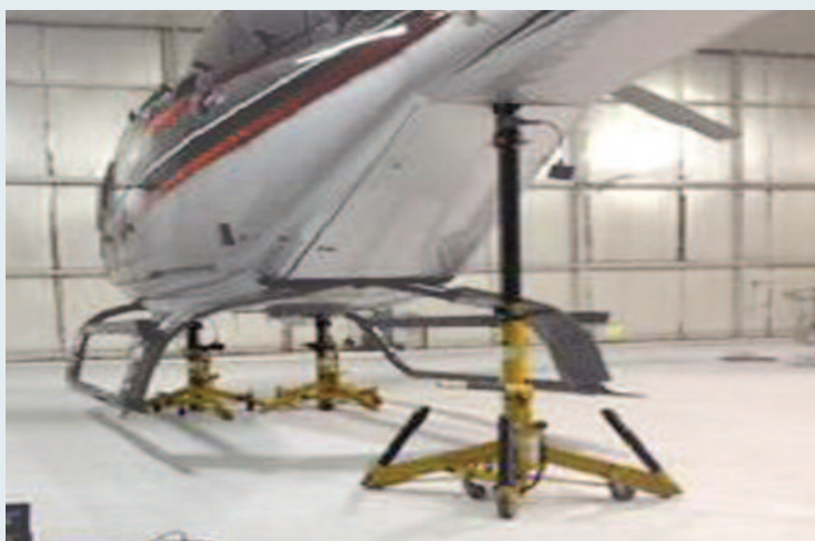
EC 120's rear (aft) lifted with the TriTask A634 Aircraft Jack and AT63448 Extension Tube.
