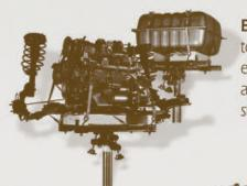
to support FWD engine/transaxle assemblies and fuel tanks. Includes struts and straps
