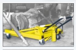
The pump can be lowered to one side, allowing the center of **TTJ** series to pass under items hanging down as much as 8-1/4" off the floor.
