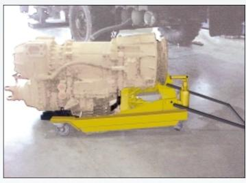
The TTJ3 Transmission Jack (NSN 4910-01-396-5044) with its new optional TTJ-Z1FA Lifting Saddle Assembly (NSN 2510-01-509-1903) easily handles the massive Allison MD 3070 PT transmission with its offset transfer case for the militarys new FMTV vehicles. Technicians can now work safely with the MD 3070 PT without being forced to remove any vehicle components or raise the FMTV.
